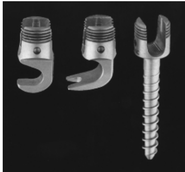
Fig. 1. — The tested implants : Standard titanium thoracic laminar hook, pedicle hook and pedicle screw (as an example a 40 mm long, 5.5 mm diameter screw).
