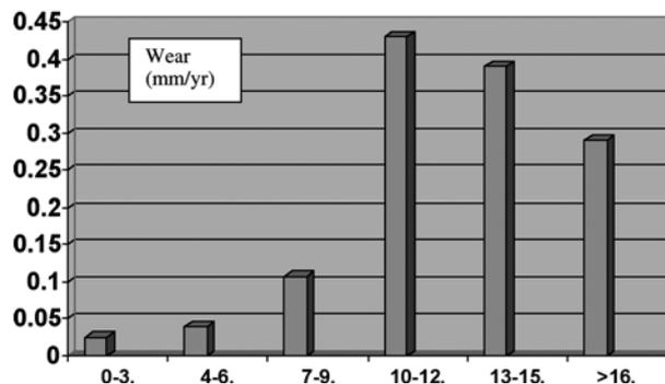
Fig. 1. — Relationship between total linear wear and time interval from production to operation (shelf life) in months.
