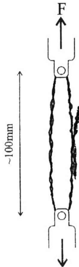
Fig. 5. — Mechanical testing of the cords.
