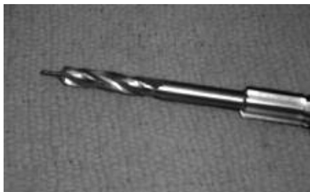
Fig. 3. — Broken wire with threads engaged in the dynamic hip screw reamer.
