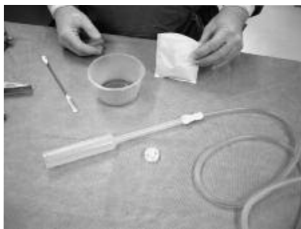
Fig. 2. — Installation with the syringe nozzle connected to the suction device.
