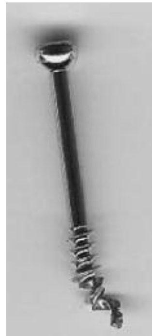
Fig. 6. — The removed screw shows unravelling – threaded area split at the troughs in a spiral configuration.
