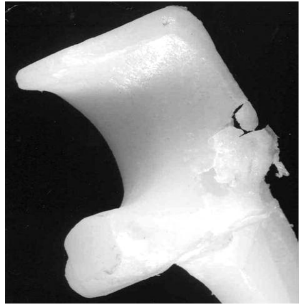
Fig. 4. — Full thickness defect in one of the ulnar components
