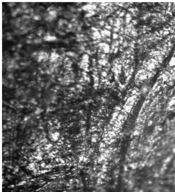
Fig. 1. — Disruption of machining lines on medial and lateral articular surfaces.
