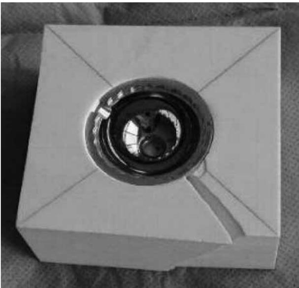
Fig. 6. — Rupture of the resin block
