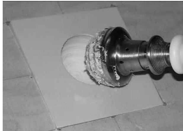
**Fig. 2.** — A 52-mm cup is impacted in a resin block after drilling at 51 mm.
