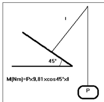
Fig. 4. — Diagram of the pull-out equipment
