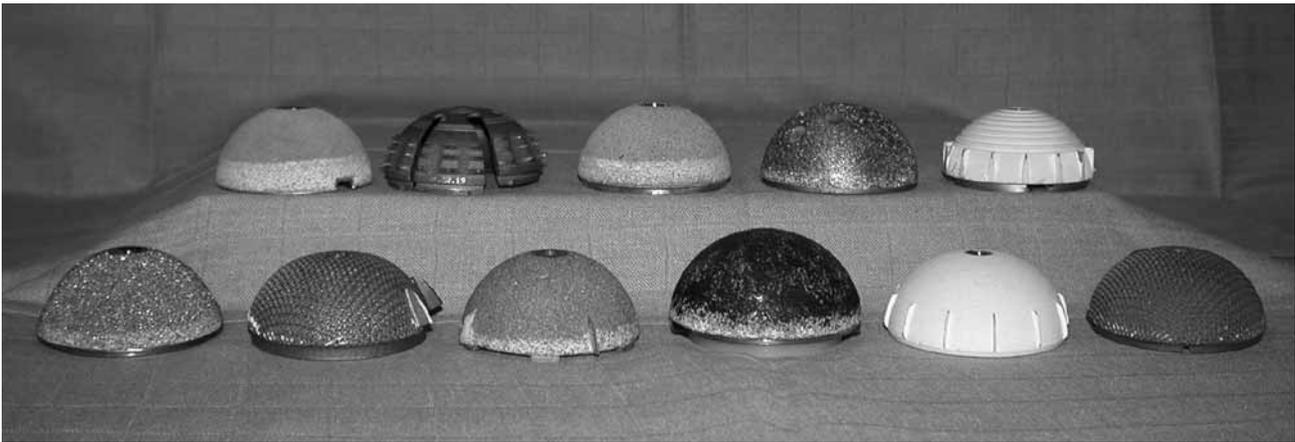
**Fig. 8.** — The larger the contact was with the resin – traces of which can be seen on the cups after pull-out –, the better was the stability.
