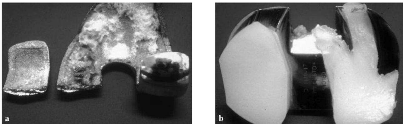
**Fig. 4.** — (a) View of the retrieved femoral component, with a fractured medial condyle at the junction between the distal part and the posterior bevel. (b) View of the retrieved tibial component, with complete wear of the posterior part of the medial polyethylene bearing while the lateral bearing is intact.
