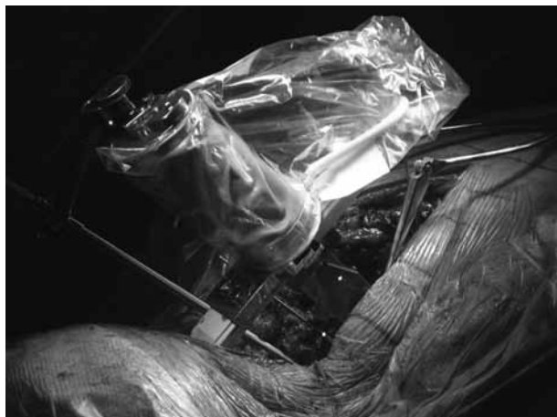
Fig. 2. —□The miniature robot mounted posteriorly for instrumentation of the upper thoracic vertebrae during a cervico-thoracic fusion procedure.
