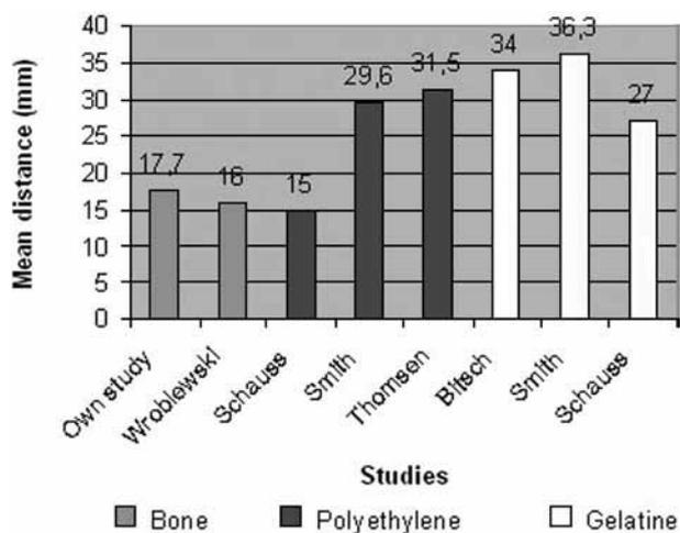
**Fig. 3.** — Overview of the mean distances between the plug and the tip of the prosthesis in studies with a comparable study design.
