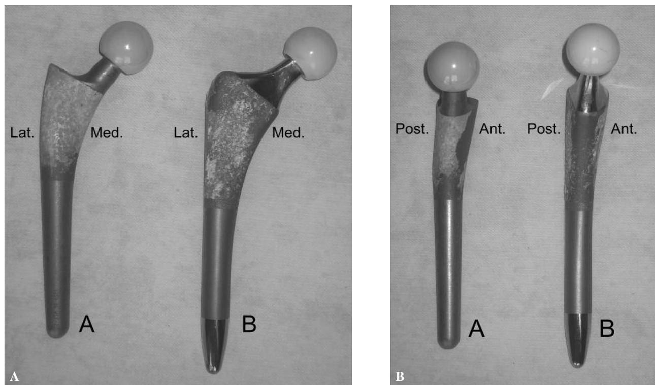
**Fig. 1.** — Profile® (DePuy Orthopaedics, Warsaw, USA) (A) and Image® (Smith & Nephew, Memphis, USA) (B) uncemented stem. Ant. = Anterior, Post. = Posterior, Lat. = Lateral, Med. = Medial. Both implants were retrieved during revision surgery and have different sizes.
