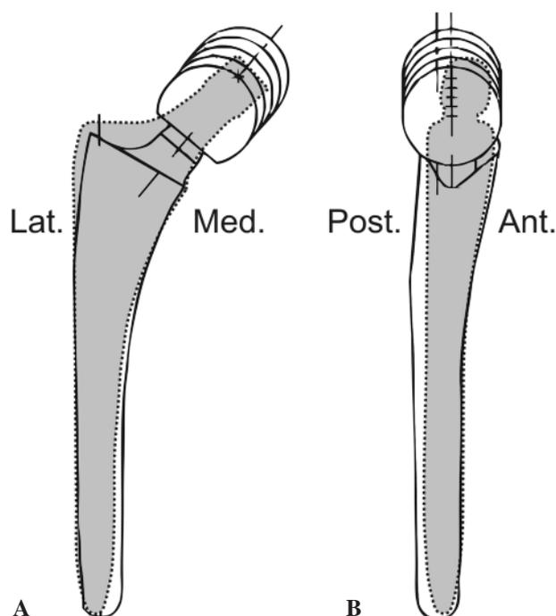
**Fig. 3.** — Superposition of the templates of a Profile® stem size 11 (white, —) and an Image® stem size 2 (gray, ....). Both stems have similar dimensions. In the AP view (A), the Image® stem is bulkier in the proximal 1/3, but not in the lateral view (B). In both views, the Image® stem is thinner distally. Ant. = Anterior, Post. = Posterior, Lat. = Lateral, Med. = Medial.
