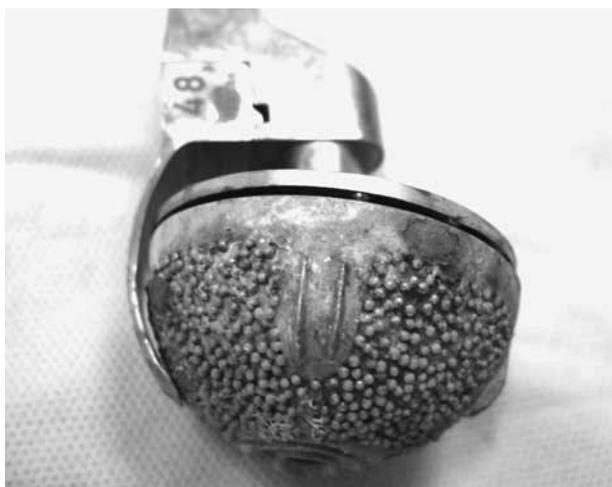
**Fig. 3.** — An explanted BHR socket with the adaptor device *in situ* showing minimal acetabular bone loss. The stabilizing fins are also shown. These are at right angles to the fixation surface.
