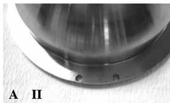
**Fig. 2A.** — (I) BHR cup adaptor device assembled to an Explant™ stem. (II) The peripheral slots for attachment to the *in situ* cup are clearly seen.
