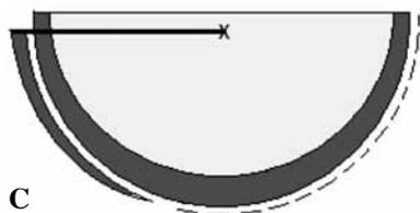
**Fig. 1C.** — When the radius of curvature is corrected by the adaptor device, the Explant™ blade passes freely around the cup.
