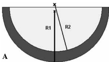
**Fig. 1A.** — The dual radius design of the BHR acetabular component. R1 illustrates the radius of the outer (fixation) surface. R2 illustrates the radius of the inner (bearing) surface.
