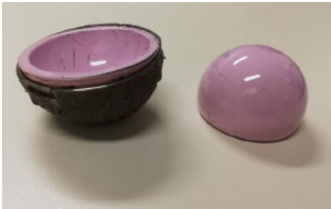
Figure 2. — Removed cup showing slight dissociation of the ceramic liner.
