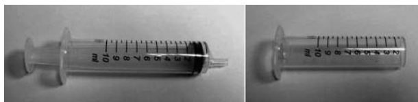
Fig. 1. — The syringe plunger has been removed and the syringe nozzle cut off with a sharp knife.
