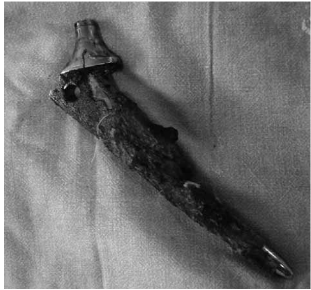
Fig. 3. — Intraoperative photograph of the retrieved implant showing fracture of the femoral neck.
