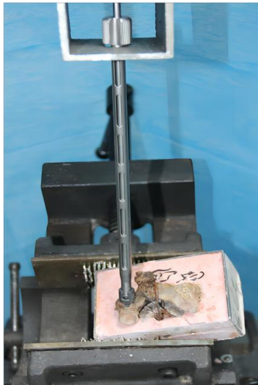
Fig. 2 — Experimental setup for evaluating screw fixation strength.
