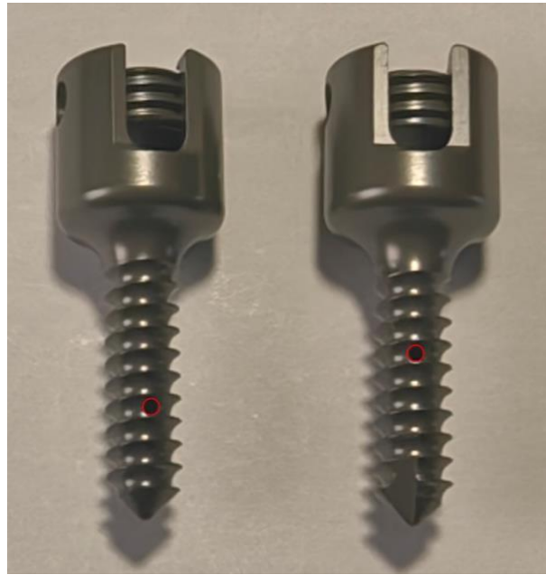
Fig. 1 — Screw design scheme. Schematic of the semi-cannulated screw, featuring side holes located 6 mm and 9 mm from the tip to enable directional cement augmentation.
