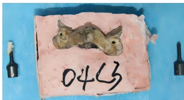
Fig. 6 — Cohesive complex formed between the screw and PMMA, accompanied by an avulsion fracture of the lateral mass.
