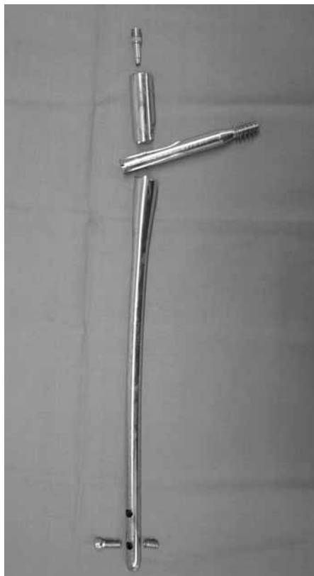
Fig. 6. — Retrieved broken nail in case 4. Showing breakage of the nail proximally and distally as well as the distal locking screw which was removed with great difficulty.
