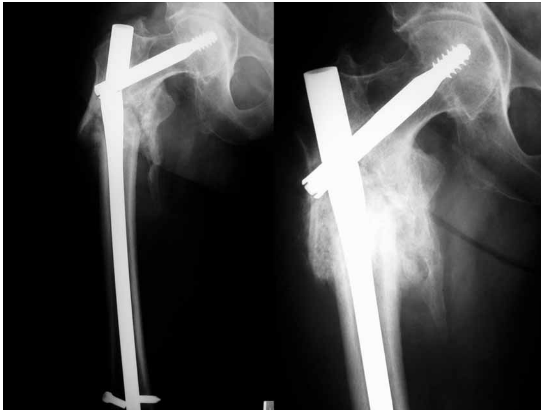
Fig. 5. — Case 4. Breakage of a long Gamma nail at the opening for the cervical screw. The distal locking screw is broken as well (left). To the right, consolidation of the fracture twelve weeks after implanting a long Gamma nail with no distal locking.
