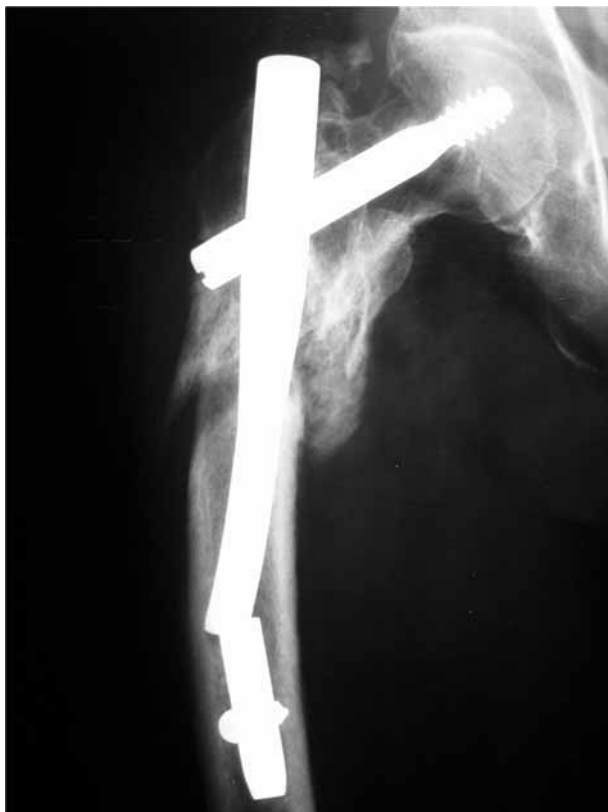
Fig. 4. — Radiological examination 8 months after implanting a Gamma nail in case 3. The nail is ruptured at one of the openings for the distal locking screws.
