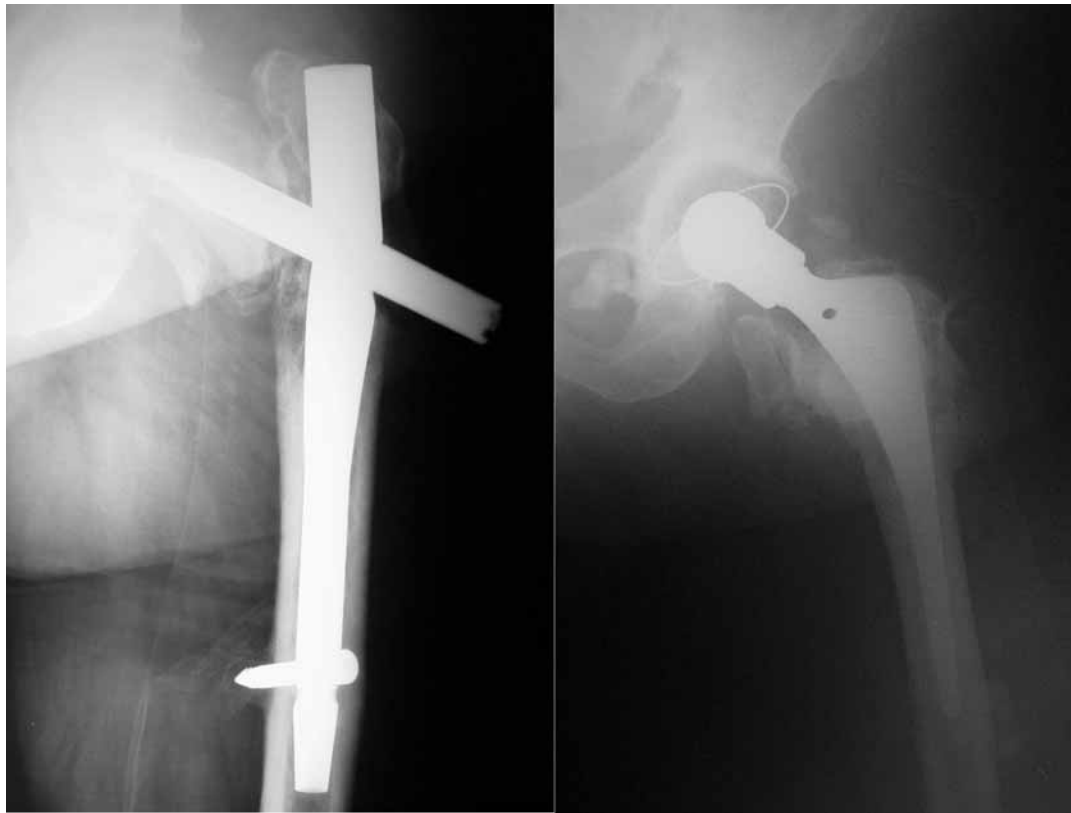
Fig. 7. — Breakage at the opening for the cervical screw in case 5. The distal locking screw is not inside the opening in the nail (left). The patient underwent a cemented total hip arthroplasty (right).
